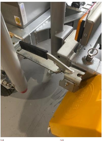
Product Details Use on current model to enhance stability when towing. Supplied as a set with Rubber Handles. Requires fitting and welding by qualified trades.
